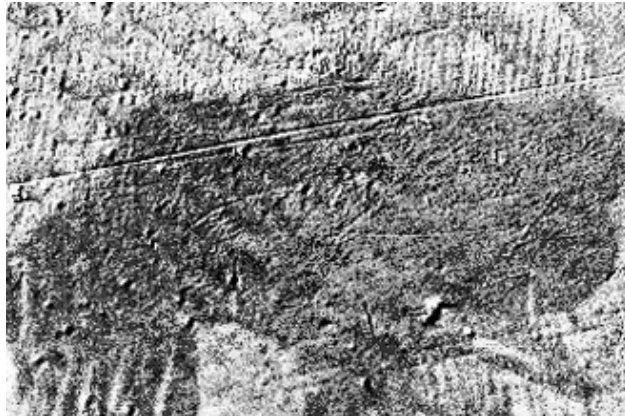
Figure 1: Optical image of a ferromagnetic domain in a silicon steel obtained by Kerr microscopy.
